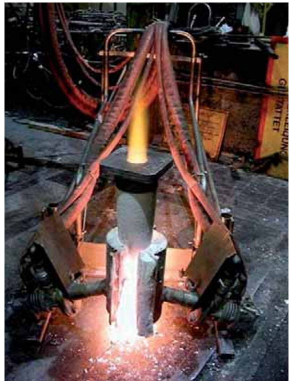
Stopper rod heating
