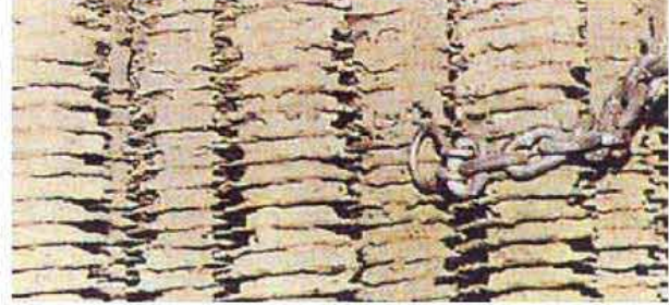
Helical finned tube after 4,000 hours operation
