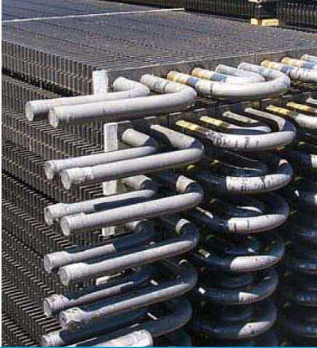
Helical finned tube after 4,000 hours operation
