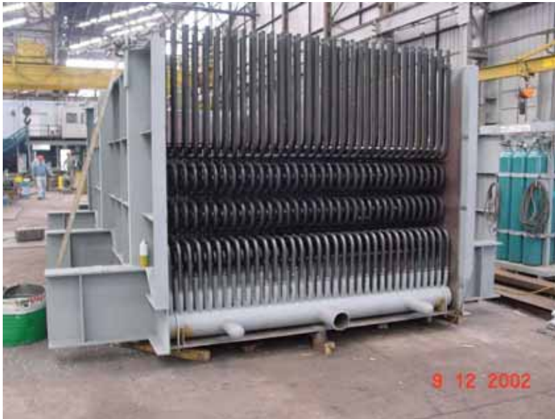
Elements installed into Casing
