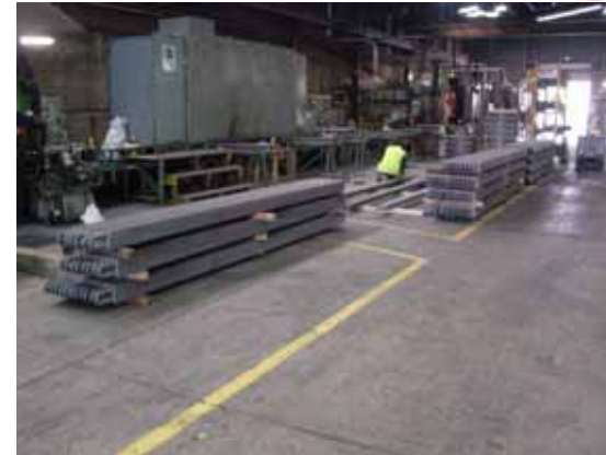
Completed Finned Tubing
