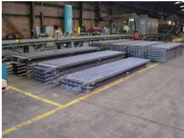
Completed Elements awaiting Hydro Testing
